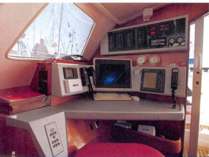
A marinized Pentium computer interfaced with Brookes and Gatehouse nav equipment, Furuno radar and GPS, and Mini-M satellite communications is at the center of the 472's nav station.
