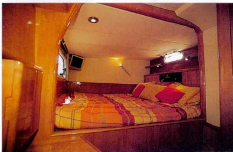
The 472's interior is a lightweight composite of cherry veneer over a foam-core sandwich. The berth is square, 6 feet 6 inches per side.
